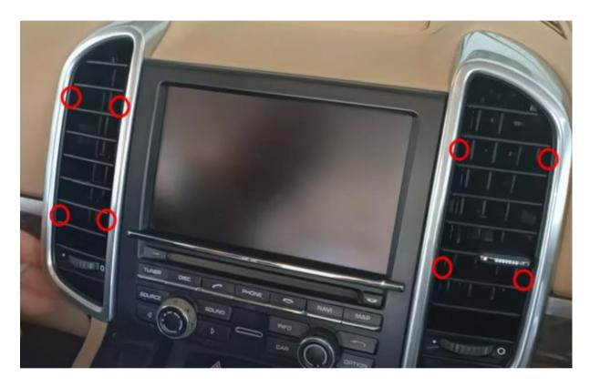
Using a flathead screwdriver, pull the 4 clips inwards and then remove the air vent. Repeat for the other air vent.
